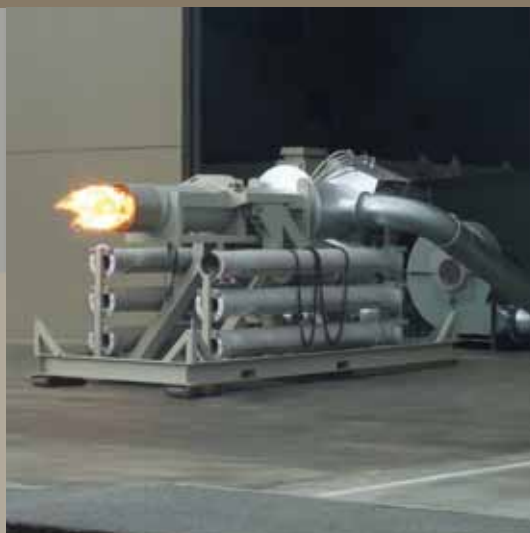
Low NOx Recirculated Combustion Gas Burner System.
